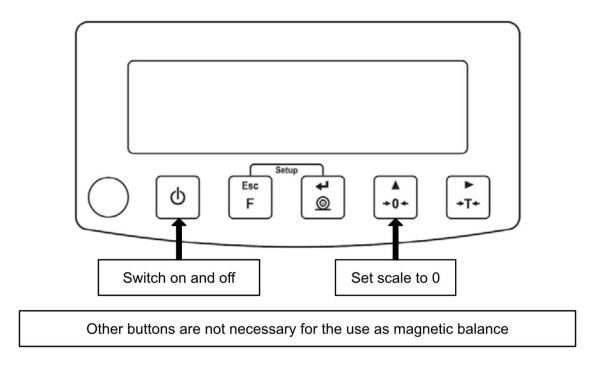
In order to zero the display, please press the "-> 0 <-" button. The zero appears at the display. The scaling to zero is only possible when the MagneticScreenScale are placed properly on the ground. Hint: The zeroing is only possible in the range of  $\pm$  2% of the maximum load. If the value is above  $\pm$  2% of the maximum load, "<Err2>" appears and an acoustic signal is given.
