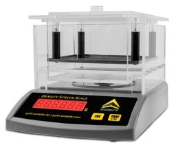
The Goldanalytix DensityScreenScale is a great device for testing precious metals of different sizes for their authenticity. Most fake coins, ingots or jewellery can be detected by using the Density Balance because of different densities of the objects. The density of gold, for example, is higher than the density of many counterfeit alloys. www.gold-analytix.com/density-balance
