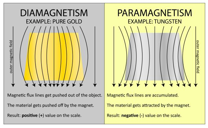
In contrast to that, **paramagnetic substances** are **weakly attracted**. Consequently, a strong magnetic field is necessary in order to gain a certain effect.
